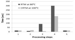
**Figure 1:** Comparison of the RTM and CRTM processing steps for the same resin system. RTM: 1. Place preform, 2.Close mould, evacuate, 3. Inject resin, impregnate, 4. Cure, 5. Demould. CRTM: 1. Place preform, 2. Inject resin, close mould, 3. Impregnate, 4. Cure, 5. Demould.
