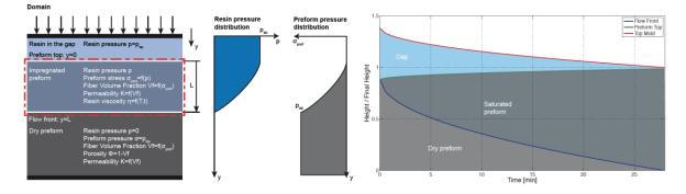
**Figure 2:** *left - description of the simulation domain; centre - evolution of resin pressure and preform pressure in the domain; right - evolution of the impregnated domain over time at constant pressure.*
